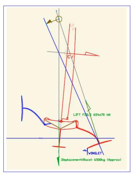
Modifying the TRIM of the Foiler by playing on the rear empennage will have very little influence on the angle of incidence (thus on the thrust produced) of the foil downwind.
