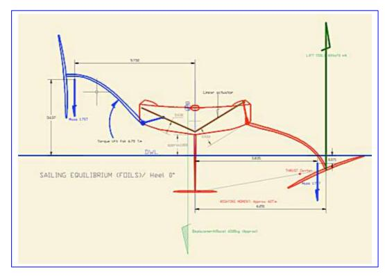
Contrary to what is said, the raised foil, which is windward, does not increase stability because there is one foil on each side (BB and TB). The resultant of the masses of these two foils is even downwind, because the lever arm of the active foil is more important than that of the raised arm!!
