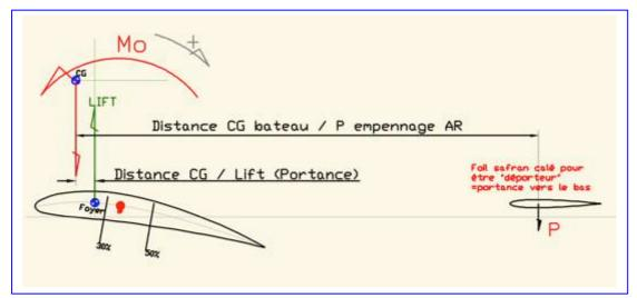
Both wings are fitted with a fixed angle of incidence relative to the aircraft body. The grey horizontal line represents a parallel to the runway. The CP Lift Centre (red point above) of a profile is the point of its cord around which the moment resulting from the aerodynamic forces applied to the profile is zero. Vertical Lift and Horizontal Drag apply at this point.
