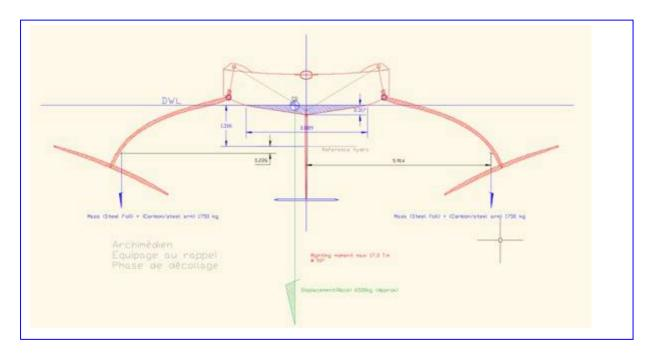
The crew is windward, which explains why the CG (Centre of Gravity is eccentric). The boat is placed in a navigation position that produces the maximum speed (approximately 16 knots) in order to reach the flight area by relying on the 2 foils. *Configuration 3 (switch from Archimedian mode to Foiler mode)*
